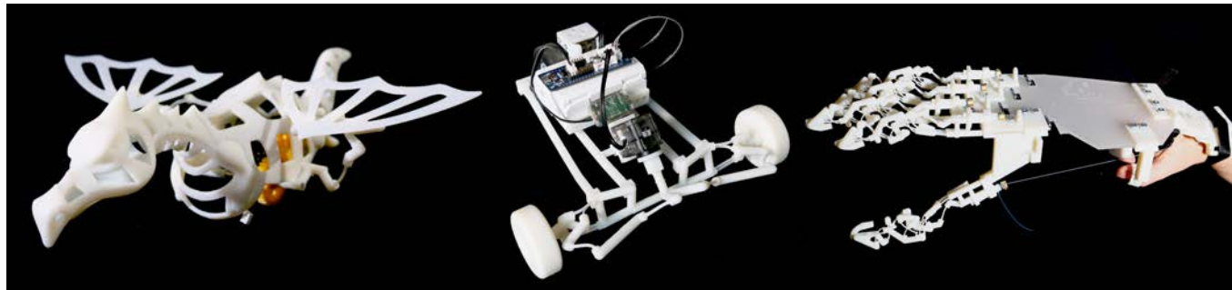
Fig. 1. Our computational tool for designing compliant mechanisms allows non-expert users to generate compliant versions of conventional, rigidly-articulated mechanisms. As we demonstrate with a diverse set of examples ranging from a spatial wing (left) and steering mechanism (middle) to a compliant hand well-suited for teleoperation tasks (right), our technique leads to structurally-sound and function-preserving compliant designs.
