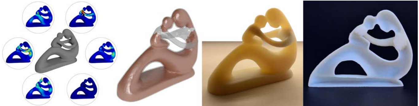
Fig. 1. We present a method for lightweight structure design for scenarios where external forces may contact an object at a multitude of locations that are unknown a priori. For a given surface mesh (grey), we design the interior material distribution such that the final object can withstand all external force combinations capped by a budget. The red volume represents the carved out material, while the remaining solid is shown in clear. Notice the dark material concentration on the fragile regions of the optimum result in the backlit image. The cut-out shows the corresponding interior structure of the 3D printed optimum.
