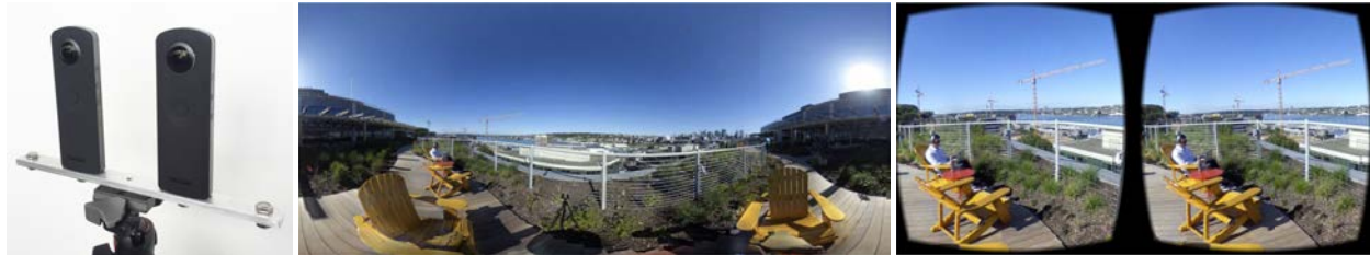
Fig. 1. (a) our stereo rig; (b) left eye equirectangular image; (c) cross-eyed stereo pair from balcony scene.
